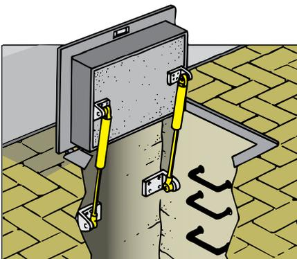
When the piston rod is pushed inside the cylinder there is less space available for the gas in the cylinder because the volume of the piston rod reduces the remaining volume inside which is occupied by the gas. Therefore, the gas pressure increases as the gas spring is compressed. This is called "progressivity of the gas spring". The increase in force usually amounts to approx. 30 % when the piston rod is completely compressed.
