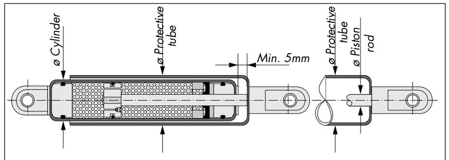
We recommend you order a protective tube when the gas spring is exposed to a high level of contamination. It also protects the piston rod from mechanical damage and therefore increases the operational life of all gas springs. Scratches, dust, dirt, paint or other damages to the surface of the piston rod cause the gas spring to wear prematurely and fail. The protection tube of AISI 304 stainless steel has the order code 9.
