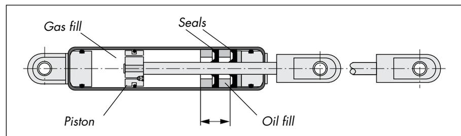
Virtually all DICTATOR gas springs are available with an additional oil chamber. This prevents the seal on the piston rod from drying out and failing. The oil also ensures easy sliding of the piston rod and reduces friction.
