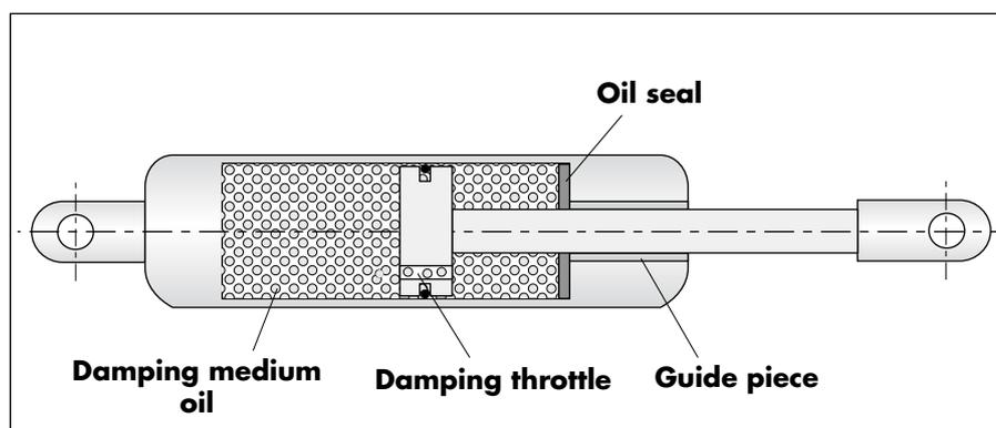
The **adjustable oil dampers with fixings on both ends (ÖDR)** use the stepped adjustment of the final dampers. The damping is adjusted by pulling and turning the piston rod.
