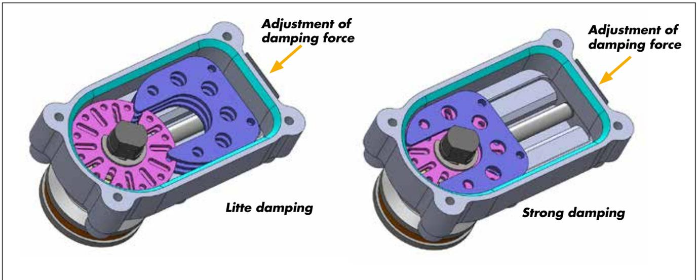
In case of the radial dampers **type RD 240/241** the damping is adjusted by an adjusting screw on the side of the aluminium casing.
